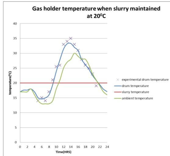
Figure 1 Gas holder temperature when slurry temperature maintained at  $20^{\circ}\text{C}$
