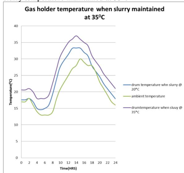
Figure 2 Gas holder temperatures when slurry temperature maintained at  $35^{\circ}\text{C}$
